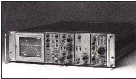
The R7903 requires only 5.25 inches of rack height in a standard 19-inch rack. It is fan-cooled and comes complete with slideout chassis tracks.
